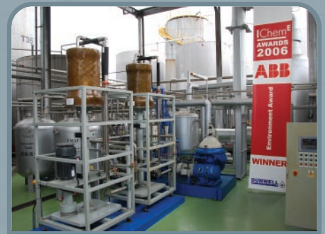
VMAT - Vibrating Membrane Used Oil Recycling System
